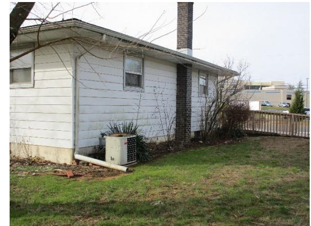
Two rain gardens can be installed to the north and south of the building to capture, treat, and infiltrate the stormwater runoff from the rooftop of the building. A preliminary soil assessment suggests that the soils have suitable drainage characteristics for green infrastructure.
