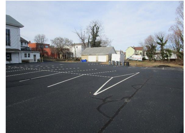
A section of parking spaces can be converted to porous pavement to capture and infiltrate runoff from the parking lot. A preliminary soil assessment suggests that the soils have suitable drainage characteristics for green infrastructure.
