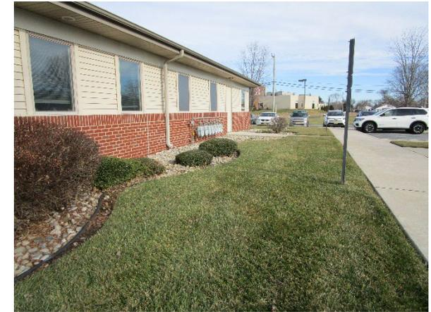
Rain gardens can be installed in the turfgrass area adjacent to the northernmost part of the parking lot and west of the southernmost building to capture, treat, and infiltrate stormwater runoff from the parking lot. Parking spaces in the northern and southern lot can be converted to porous pavement to capture and infiltrate stormwater runoff. A preliminary soil assessment suggests that more soil testing would be required before determining the soil's suitability for green infrastructure.
